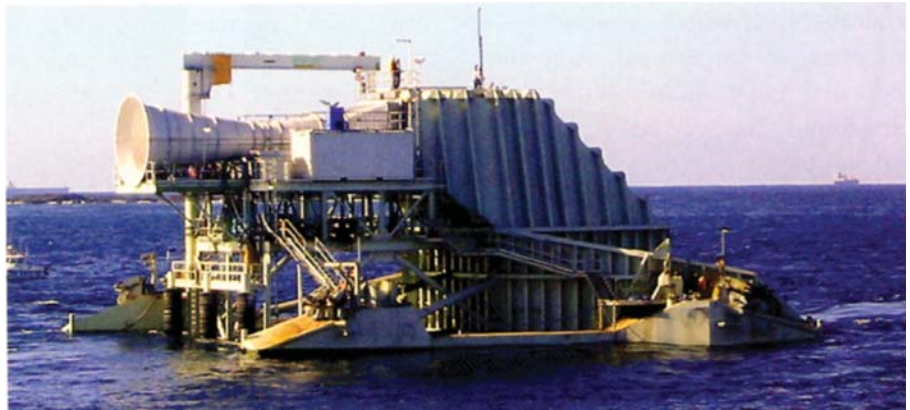
A 500-Kw wave energy conversion device being installed in the ocean near Port Kembla, Australia, should produce enough electricity to power as many as 500 homes each year.
